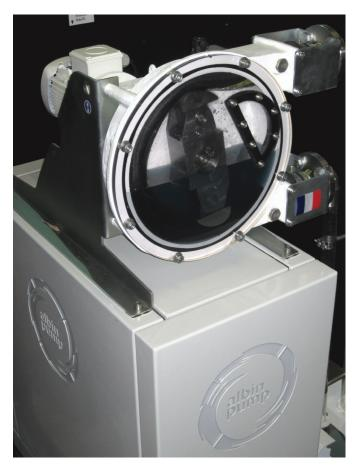
ALBIN PUMP can offer food grade hoses in EPDM FDA, NBR FDA and NR FDA and meet the certifications **EC 1935/2004 and FDA CFR21§177.2600.** The internal of the hose is white (NR FDA and EPDM FDA) or black (NBR FDA), according to the pumped fluid.
